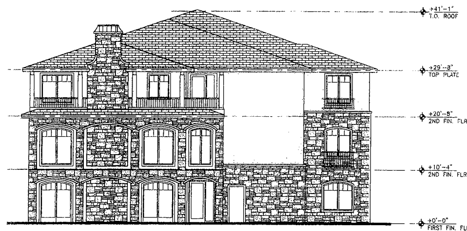
3 BUILDING "B" EAST ELEVATION SCALE: 1/8" = 1'-0" (BUILDING "C" SIMILAR)
