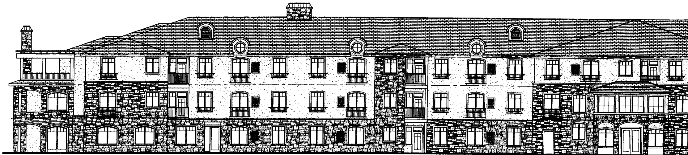
1 BUILDING "B" NORTH ELEVATION (EAST END) SCALE: 1/8" = 1'-0" (BUILDING "C" SIMILAR)
