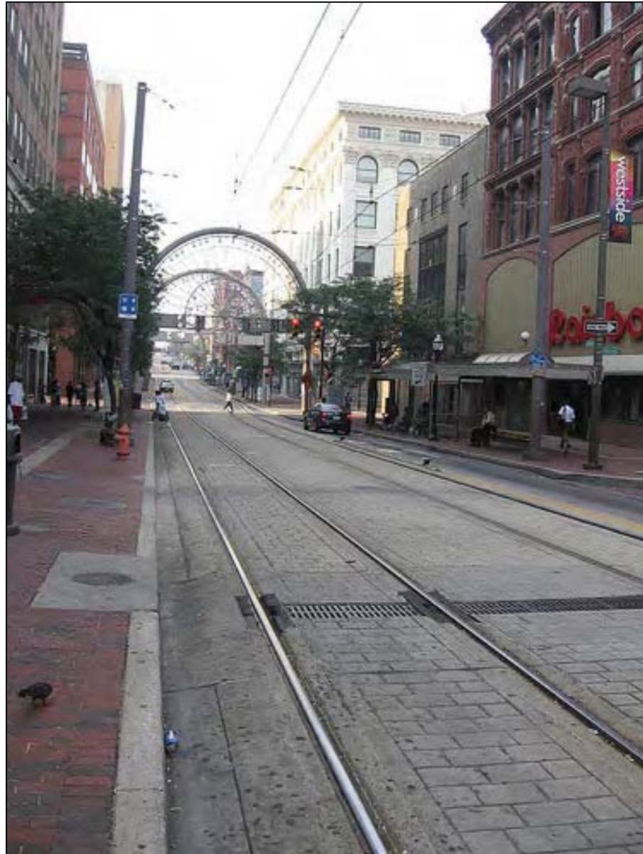
Baltimore – Pavers in light rail lanes with unique catenary system.
