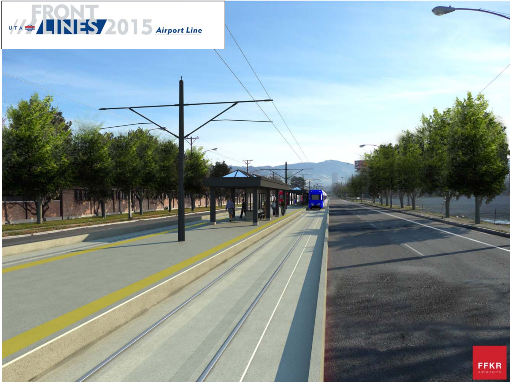
Artist's Rendering of Concrete-Embedded Tracks on North Temple
